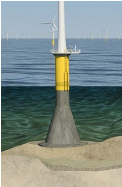
Figure 8. Gravity foundation. Illustration COWI
