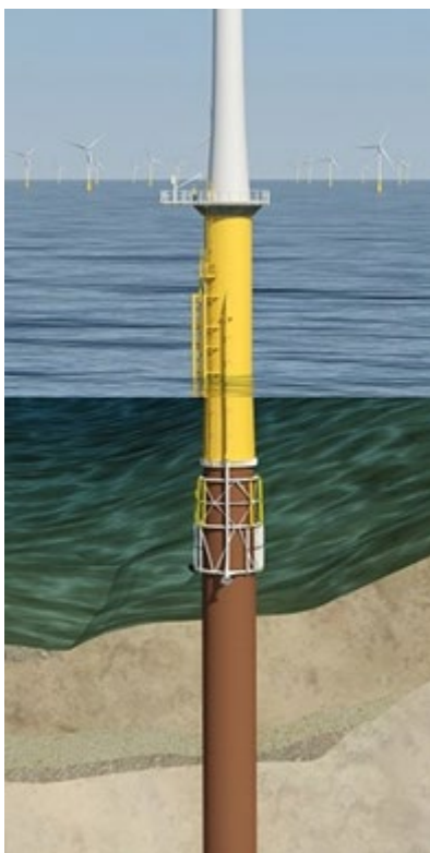
Figure 9. Monopile foundation. Illustration COWI
