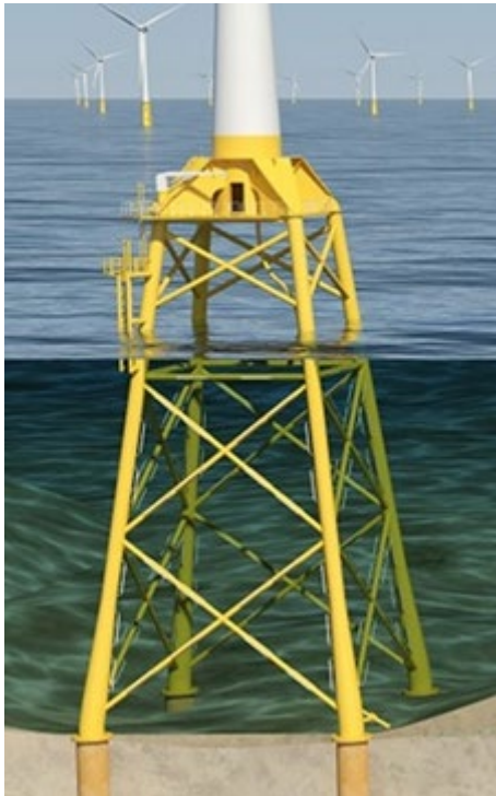
Figure 10. Jacket foundation. Illustration COWI
