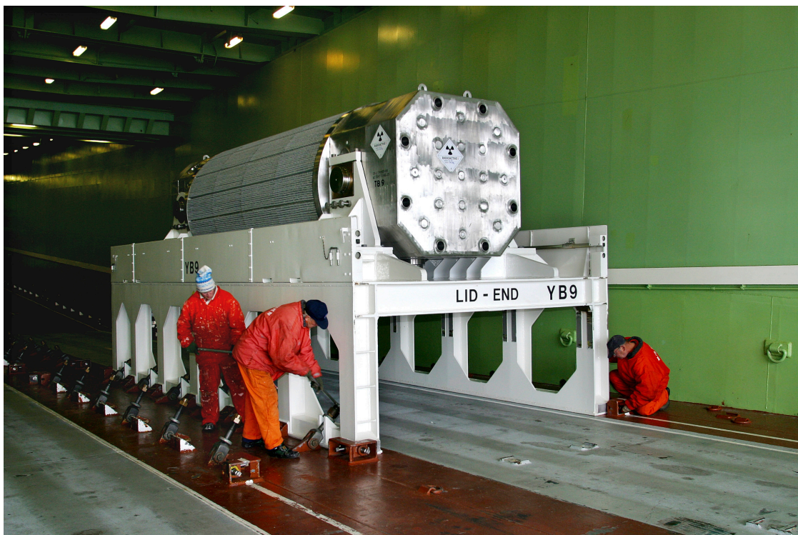
Figure 6-2. Lashing of casks for spent nuclear fuel on m/s Sigyn.
