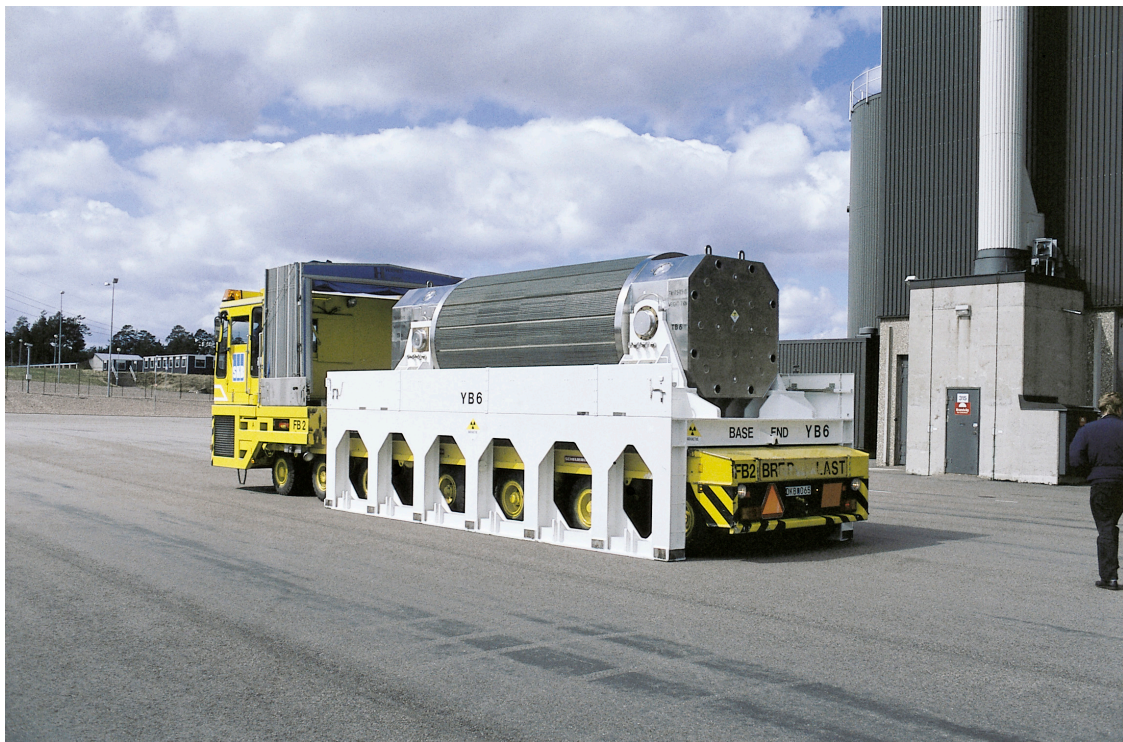
Figure 6-1. Terminal vehicle with transport cask for spent nuclear fuel.
